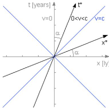
Fig. 1.2 Space-time diagram for a resting and a moving observer
