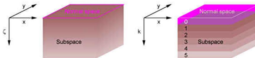
Fig. 3.1 Continuous (left) and discrete (right) subspace model
